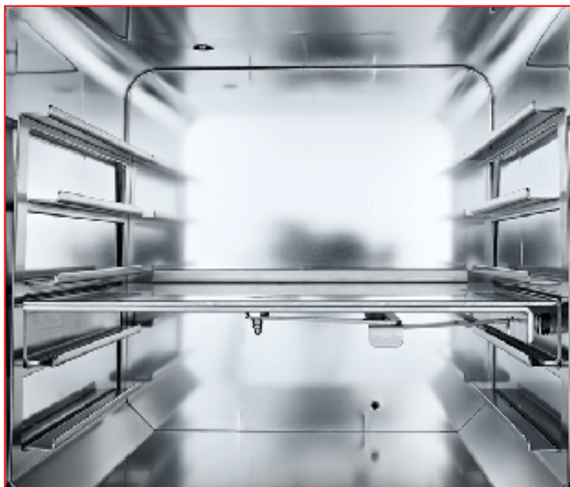
Chrome-plated racks will enable you to dry test specimens homogeneously on several levels.
