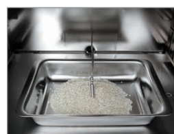
Specimen temperature display with PT 100 sensor
