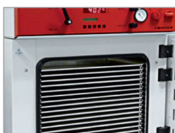
Vacuum drying oven with special racks for large numbers of particularly flat samples
