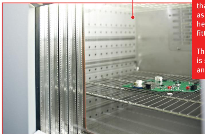
The stainless steel interior is no problem to clean and the test chamber can be loaded and unloaded with ease thanks to the prioritization of width over depth as far as the units are concerned. You can look through the heated window to check on samples and the interior is fitted with LED illumination.
