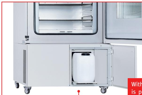
With environmental simulation chambers from BINDER, the water supply is provided independent of location via a storage tank. Humidity is regulated using a capacitive humidity sensor and steam humidification. There is also a condensation protection system you can program to further guarantee the quality of your measured data.
