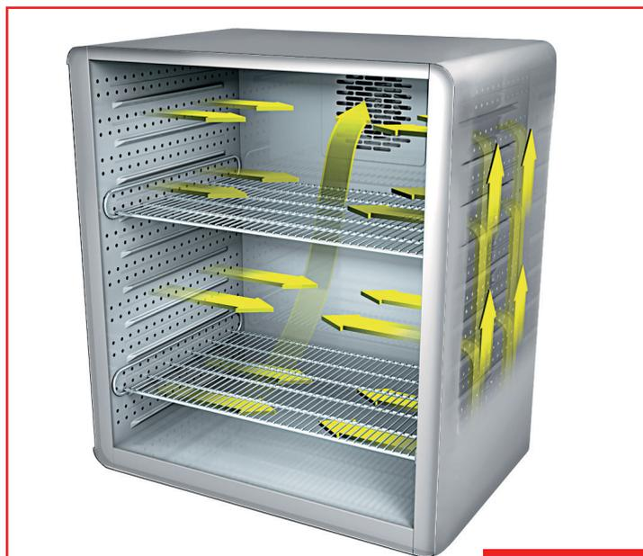
All BINDER environmental simulation chambers feature the proven APT.line™ preheating chamber technology, which ensures homogeneous temperature distribution and guarantees accurate measured values at every temperature setting. At the same time, the “Advanced Preheating Technology” provides exceedingly fast cooling down rates.
