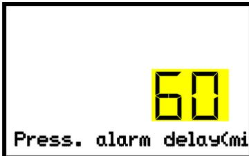
Setting the delay for pressure tolerance range alarm.
