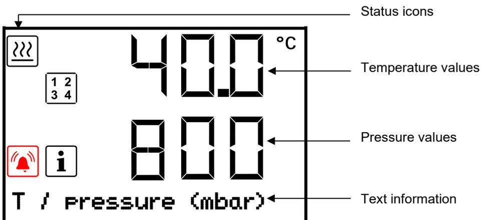
Figure 18: Normal display of the RD4 controller (sample values)
