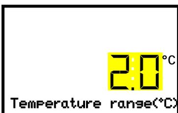
Setting the temperature tolerance range
