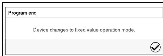
After the end of the program the message “Device changes to fixed value operation mode” appears on the screen.
