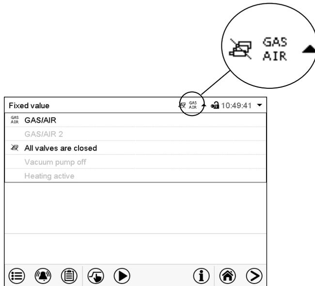
Normal display showing the text information. The currently valid information texts are highlighted in black (example: "All valves are closed" and "GAS/AIR")
