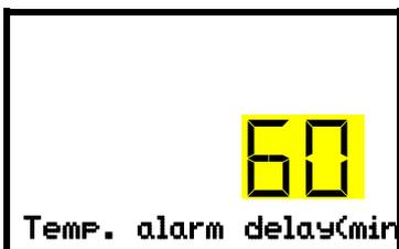
Setting the delay for temperature tolerance range alarm.
