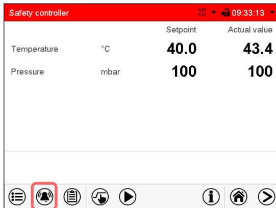
Normal display in state of alarm (example).
