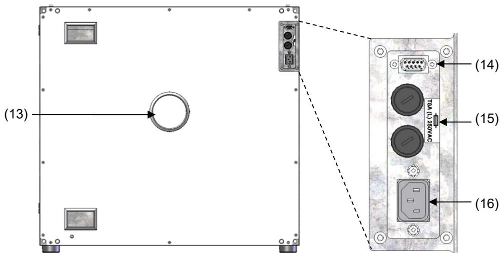
Figure 14: Pump module, rear view with connection panel (example: size 115)
