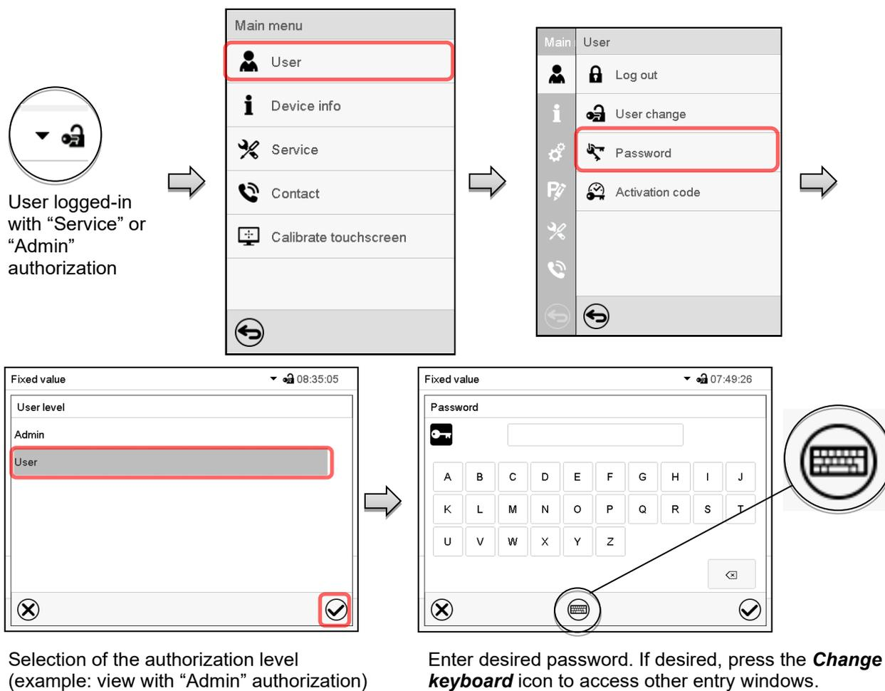
In the “Keyboard switch” window you can select different keyboards to enter uppercase and lowercase letters, digits, and special characters. All types of characters can be combined within one single password.
