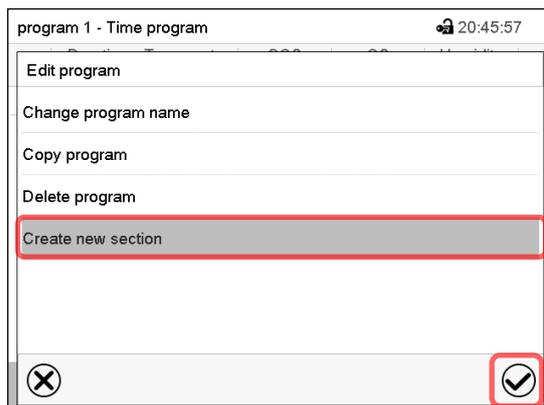
To add a new section, select "Create new section" and press the **Confirm** icon.
