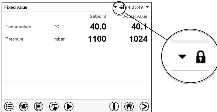
In the locked view the controller provides all display functions. No setting functions are available.
