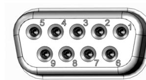
Figure 26: Sub D socket (9) “Object temperature input” in the VD rear control panel to connect the optional Pt 100 sensor
