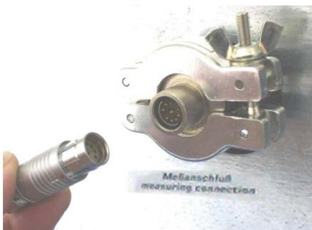
Figure 25: Measuring connection (12) with measuring access port
