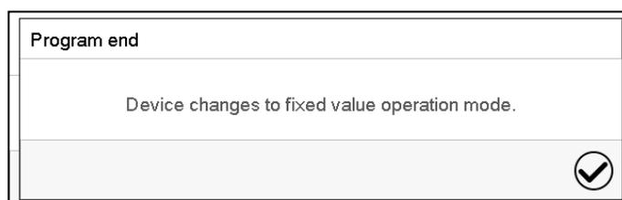
After the end of the program the message "Device changes to fixed value operation mode" appears on the screen.
