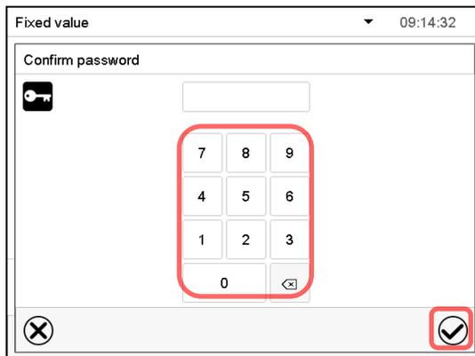
Repeat the password entry for confirmation (sample picture). For each character of the password, the required keyboard appears automatically.
