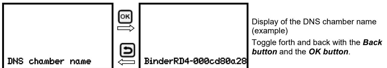
Display of the DNS chamber name (example)
