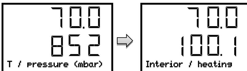
Press down the **Back button** again for 5 seconds to terminate the indication.
