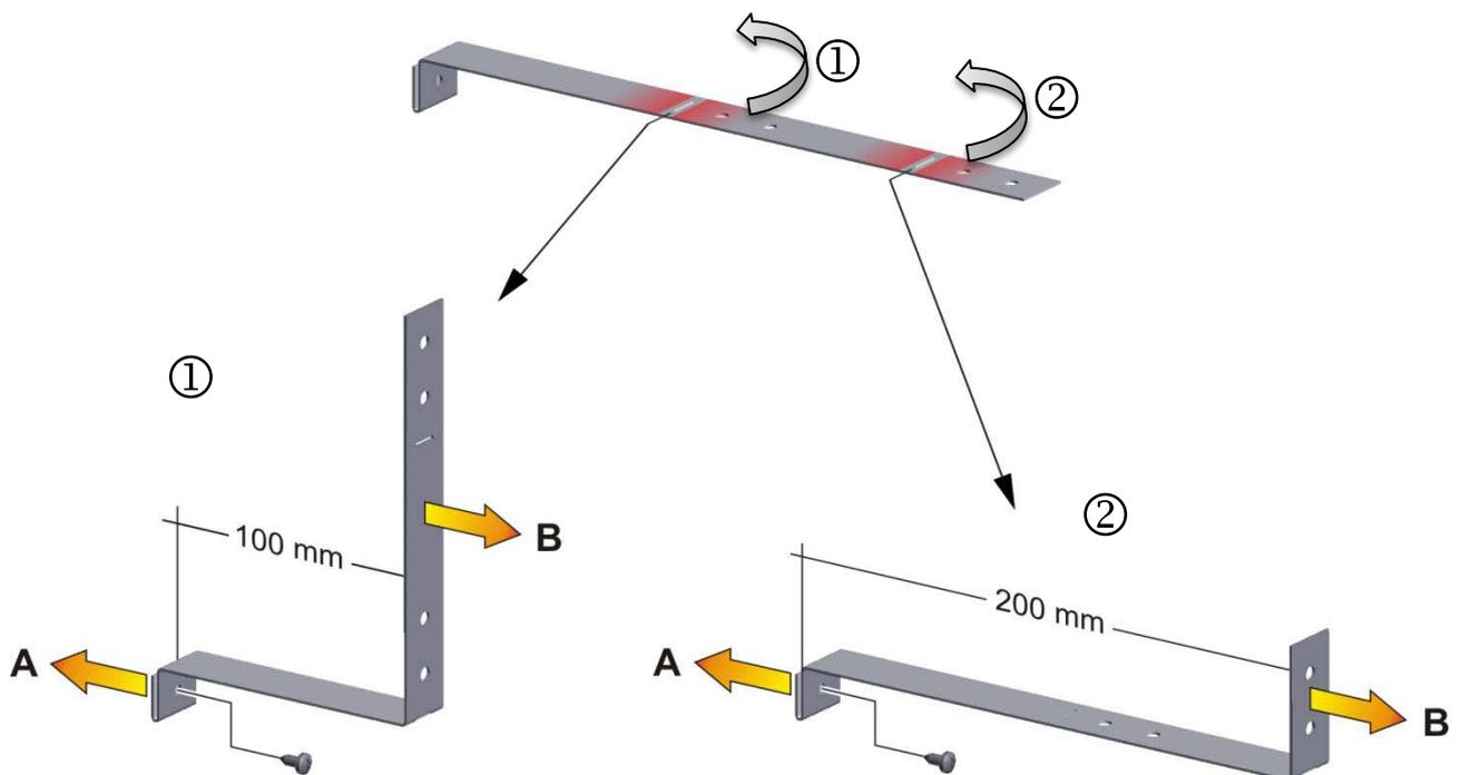
Figure 12: Variable length of the tilt protection holder depending on the bend
