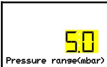
Setting the pressure tolerance range
