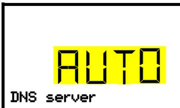
Selection of the type of assignment of the DNS server address.
