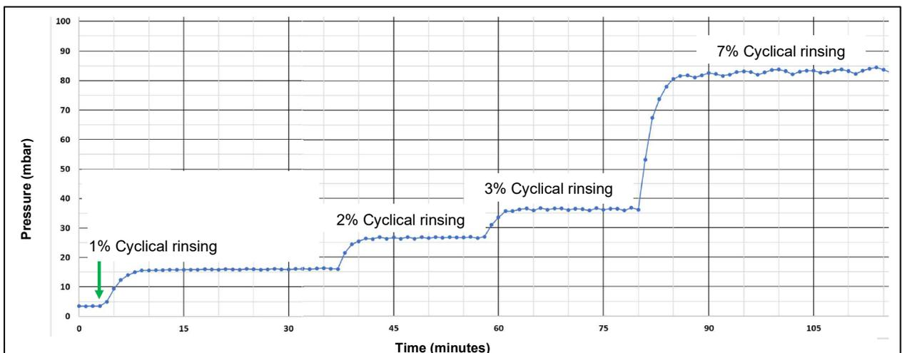
Figure 22: Pressure curve depending on the setting values for cyclic rinsing, sample representation beginning at the final vacuum of 4mbar VD 56 with VAP 2
