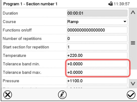
Section view, showing the temperature tolerance range
