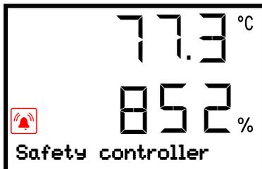
Alarm indication (example: safety controller alarm)
