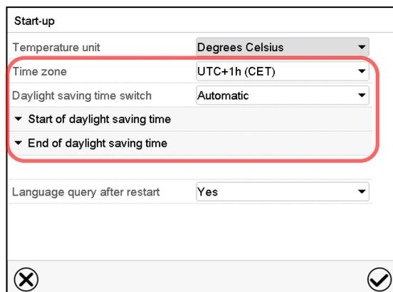
The screenshot shows the 'Start-up' submenu with the following settings: Temperature unit: Degrees Celsius; Time zone: UTC+1h (CET); Daylight saving time switch: Automatic; Start of daylight saving time: (dropdown); End of daylight saving time: (dropdown); Language query after restart: Yes. A red box highlights the Time zone, Daylight saving time switch, and the Start/End of daylight saving time dropdowns.
