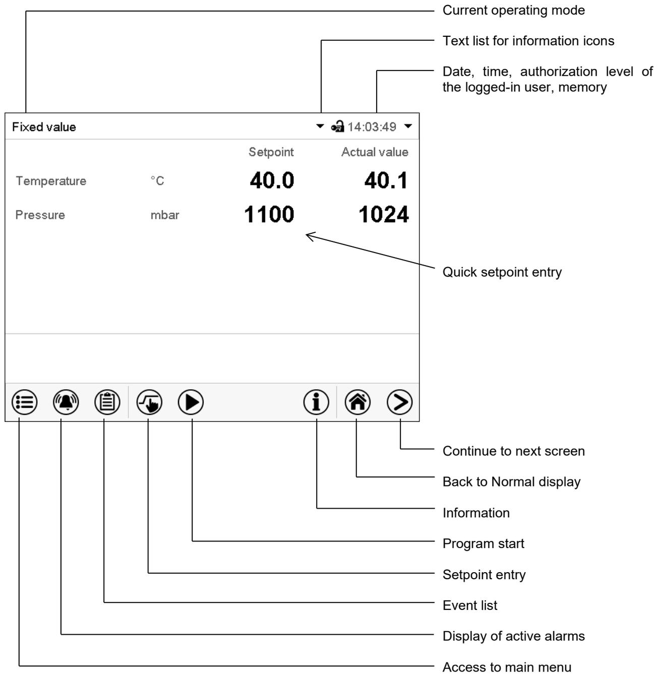
Figure 20: Operating functions of the MB2 controller in normal display (example values)
