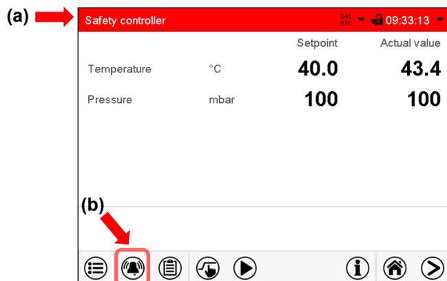
Normal display in state of alarm (example).
