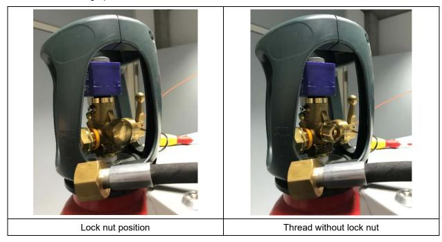
Figure 35: Lock nut in the valve
