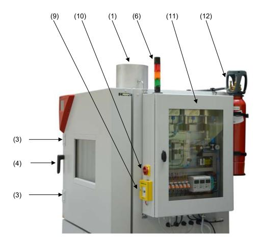
Figure 5: Front right view with safety equipment (example LIT MK 240)
