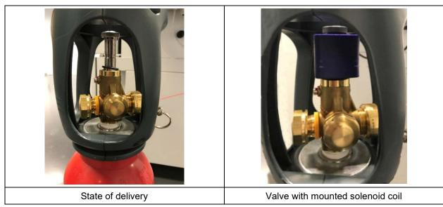
Figure 30: Valve of the CO<sub>2</sub> pressurized gas cylinder
