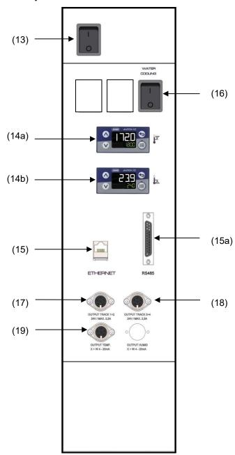
Figure 7: Lateral control panel at the right side of the refrigerating machine, with options
