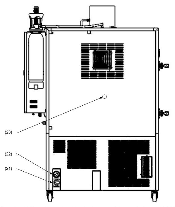
Figure 10: LIT MK rear chamber view with optional compressed air connection (example: LIT MK 240)
