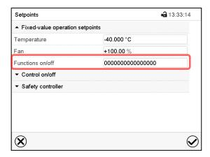
"Setpoints" submenu in fixed value operation. Select the field "Functions on/off".
