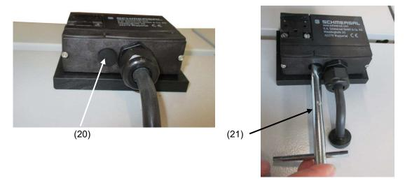
Figure 42: Mechanical emergency release
