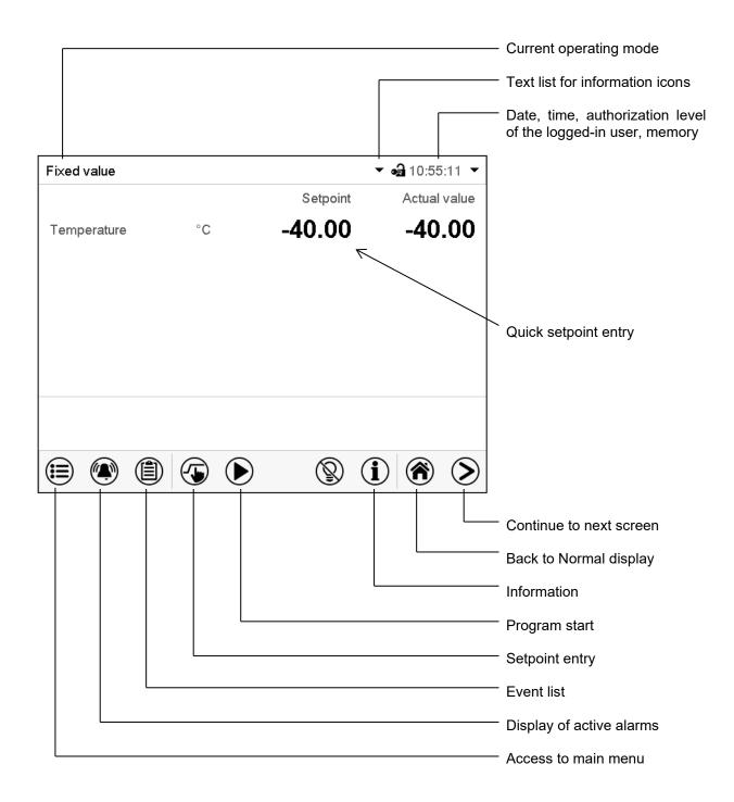
Figure 29: Operating functions of the MB2 controller in normal display (sample values)
