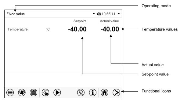
Figure 28: Normal display of the MB2 program controller (sample values)
