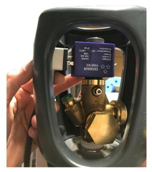
Figure 37: Connecting / disconnecting the coil connector
