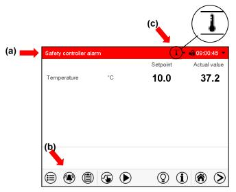
Normal display in state of alarm (example).
