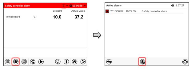
Normal display in state of alarm (example).
