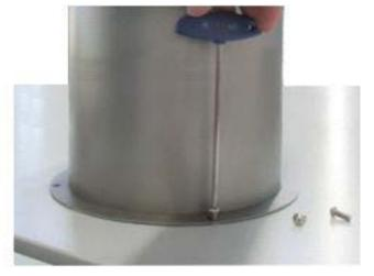
Figure 22: Mounting the exhaust port at the top of the chamber
