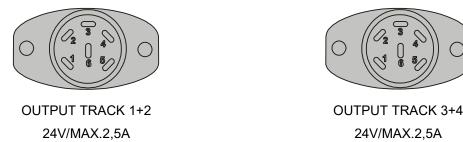
Figure 40: Pin configuration of DIN sockets (17) left and (18) right
