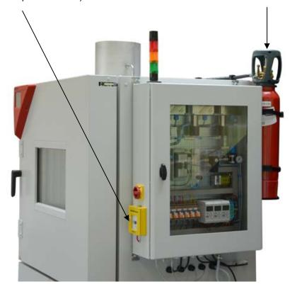
Figure 13: Location of the devices for the CO<sub>2</sub> fire suppression device
