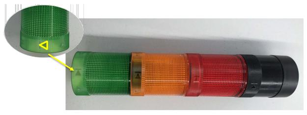
Figure 18: Indicator light (delivery condition)
