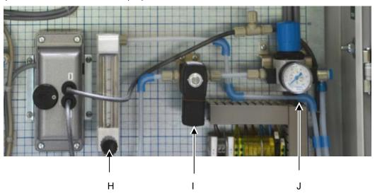
Figure 23: Inertization device components in the safety module
