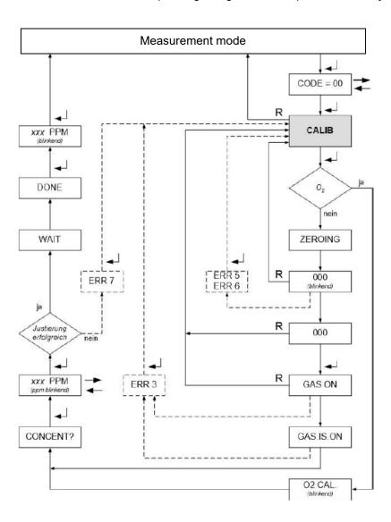
Figure 43: CALIB service menu for zero point calibration and sensor adjustment
