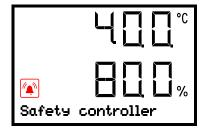
Alarm indication (example: safety controller alarm)
