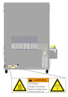
Figure 2: Position of label on the chamber rear
