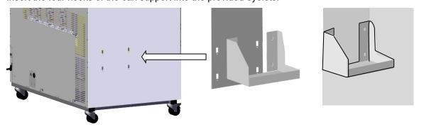
Figure 12: Attaching the can support on the left sidewall
