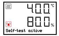
Display showing the running self-test in Normal display (example values)
