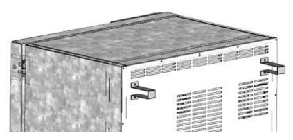
Figure 9: Rear chamber with mounted spacers
