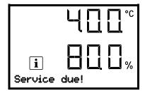
The message "Service due!" is shown in the text field of the controller display.
