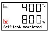
Display showing the completed self-test in Normal display (example values)
