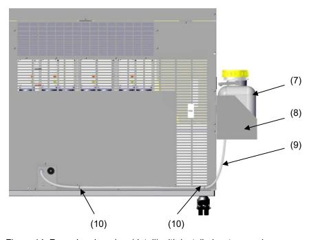
Figure 14: Rear chamber view (detail) with installed water supply
