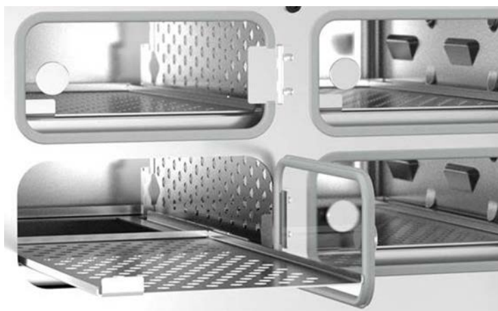
Figure 26: A look inside an incubator with the "Divided inner door with cell therapy compartmentation" option
