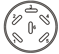
Figure 40: Pin configuration of the DIN socket (3) on the chamber rear
