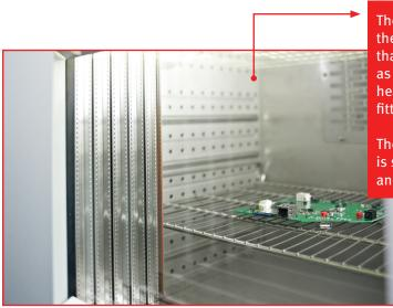
The stainless steel interior is no problem to clean and the test chamber can be loaded and unloaded with ease thanks to the prioritization of width over depth as far as the units are concerned. You can look through the heated window to check on samples and the interior is fitted with LED illumination.
