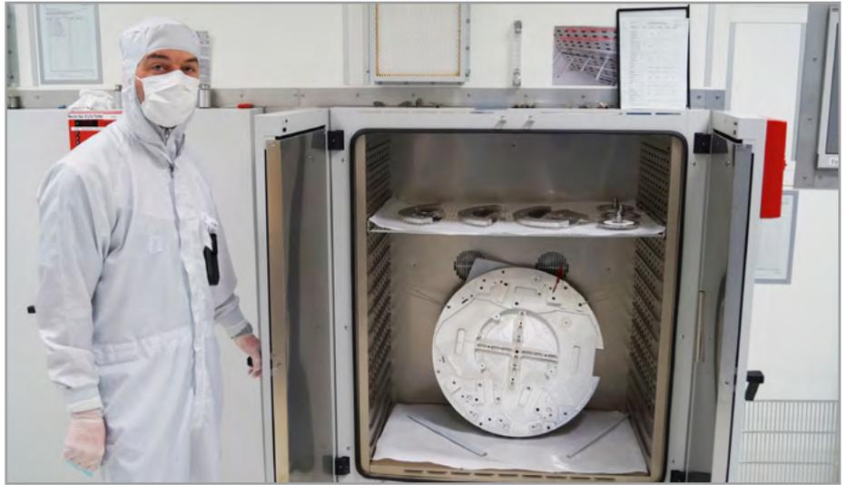
> Components that are used for producing chips must be delivered in an absolutely clean state. BINDER chambers help ensure that every last bit of liquid is removed from the pores.
