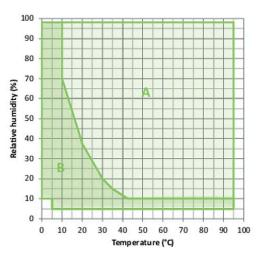
A: Standard Climate range B: Expanded range with controlled dry-air purge
