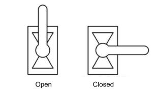
Figure 13: Lever positions of drain valve (15) for waste water connection (14)
