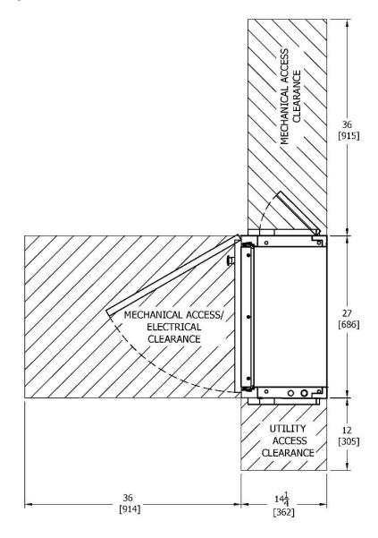
Figure 10: Required free space for access to the conditioner
