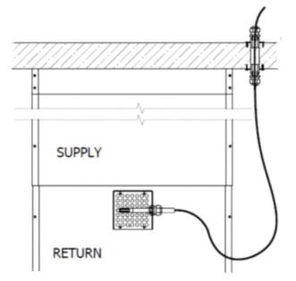
Figure 16: Installing the temperature/humidity sensor (example view)
