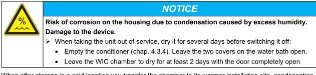
When after storage in a cold location you transfer the chamber to its warmer installation site, condensation may form. Before start-up, wait at least one hour until the chamber has attained ambient temperature and is completely dry.
