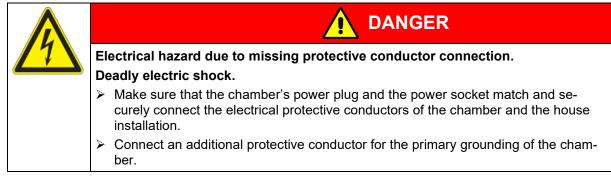
• Check the power supply voltage before connection and initial commissioning. Compare the values with the data on the type plate of the environmental walk-in chamber WIC (chap. 1.5).
