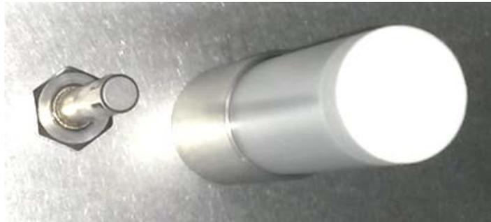
Figure 11: Plugged-in CO<sub>2</sub> sensor (right) and gas mixing head for CO<sub>2</sub>
