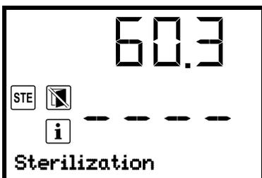
Normal display during sterilization (example during heating up phase)
