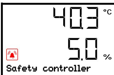
Alarm indication (example: safety controller alarm)
