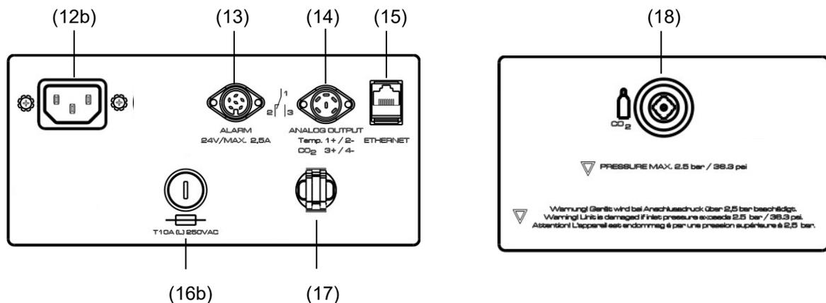
Figure 9: Rear control panel CB-S-UL with options
