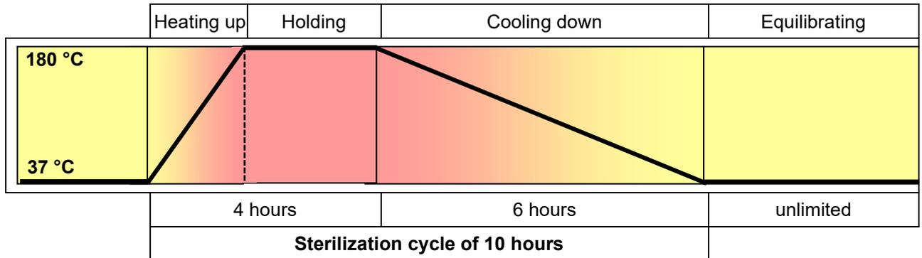
Figure 22: Setpoint profile during the sterilization cycle
