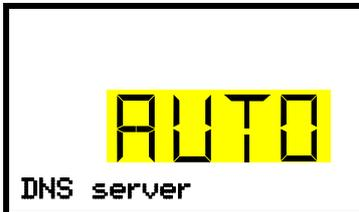
Selection of the type of assignment of the DNS server address.
