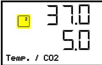
Normal display with deactivated CO<sub>2</sub> control (sample values)
