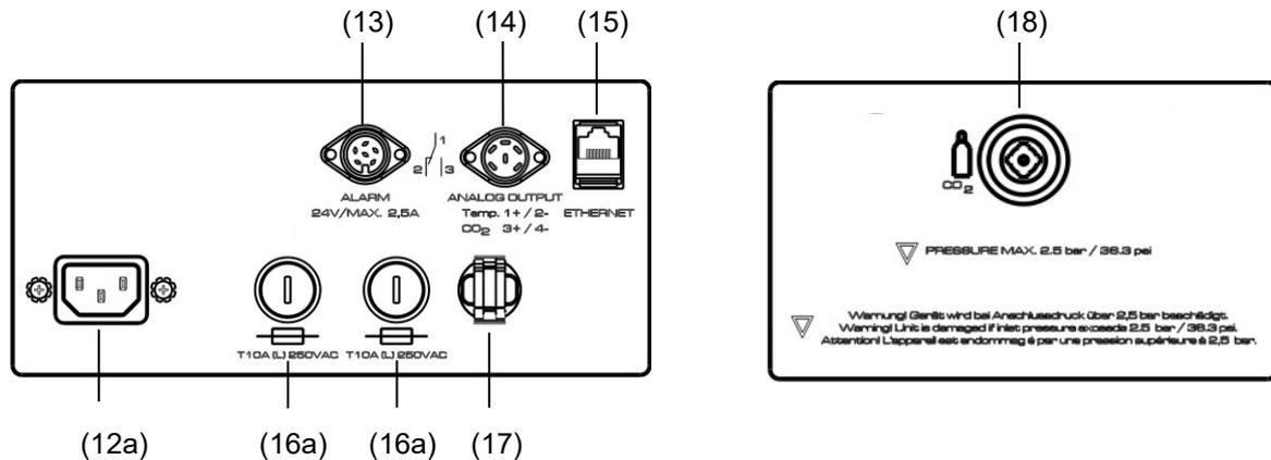
Figure 8: Rear control panel CB-S with options
