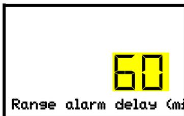
Setting the tolerance range alarm delay.
