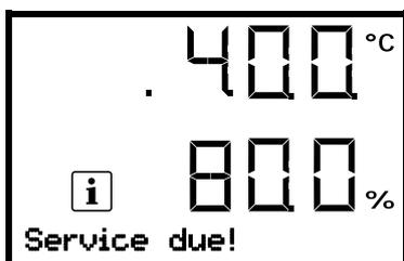
The information message "Service due!" is shown in the text field of the controller display.
