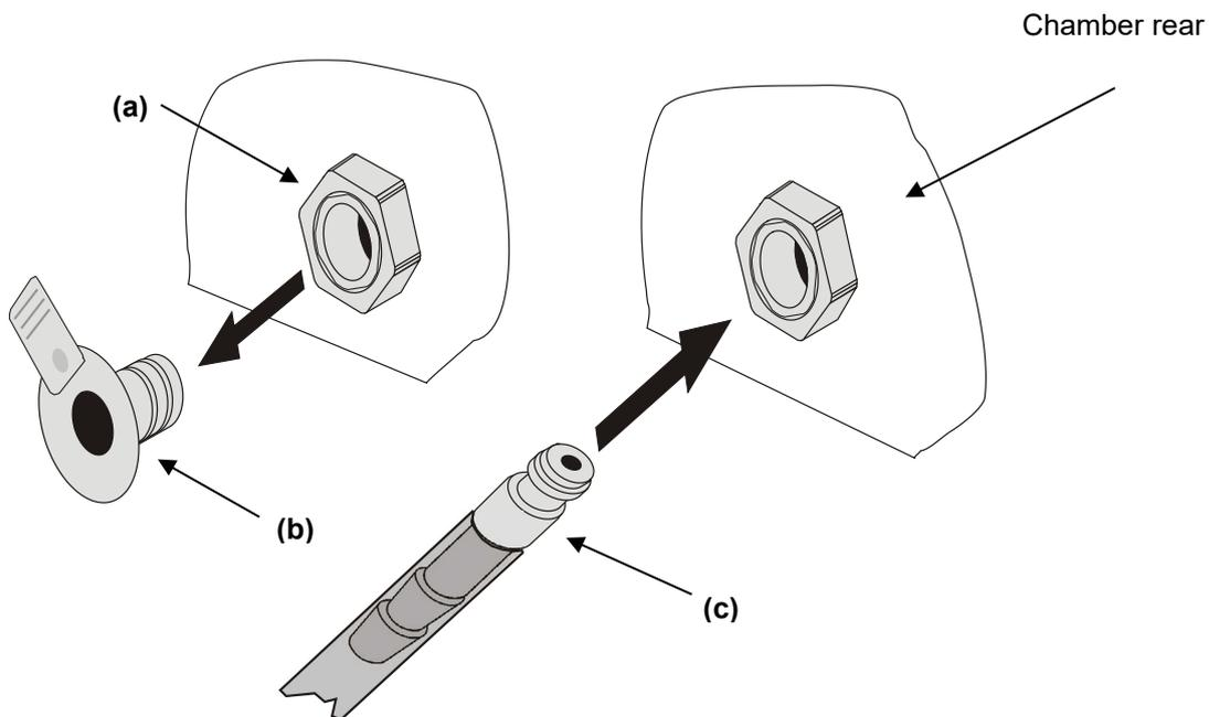
Figure 13: Connection of the hose lead to the gas cylinder
