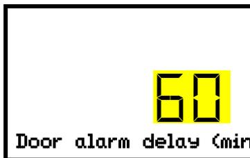
Setting the door open alarm delay.
