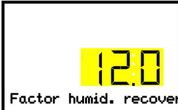
Setting the heating power factor for humidity recovery time.
