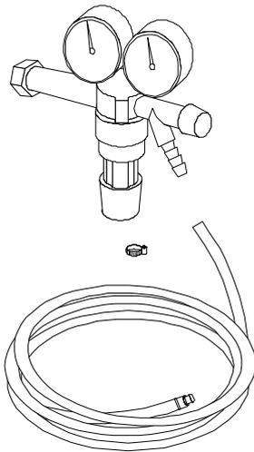
The gas cylinder connection kit for CO<sub>2</sub> (Art. no. 8012-0014) includes the following parts for connecting a gas cylinder to the CO<sub>2</sub> incubator:
