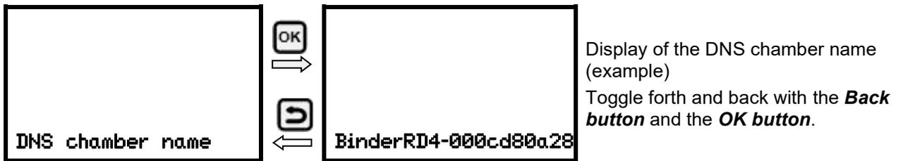
With the **Back button** you can go back to the “**Ethernet**” submenu and, repeatedly pressing it, to **Normal display**.
