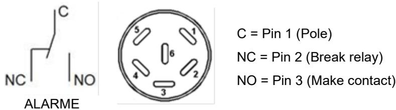
Figure 16: Zero-voltage contacts circuit diagram and pin allocation of DIN socket (13)
