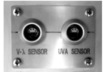
Figure 14: Lemo sockets to connect the light sensors
