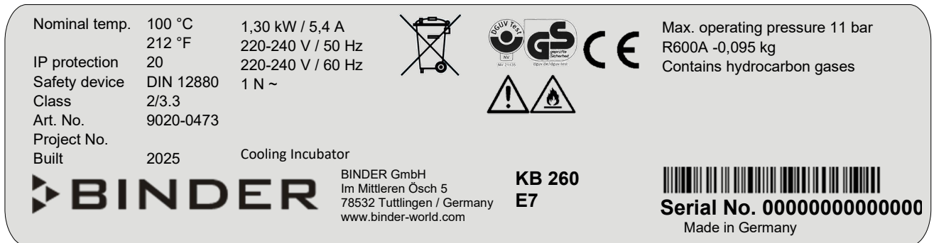
Figure 1: Type plate (example KB 260 regular chamber 9020-0473)
