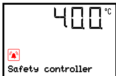
Normal display showing overtemperature safety controller alarm (sample values)
