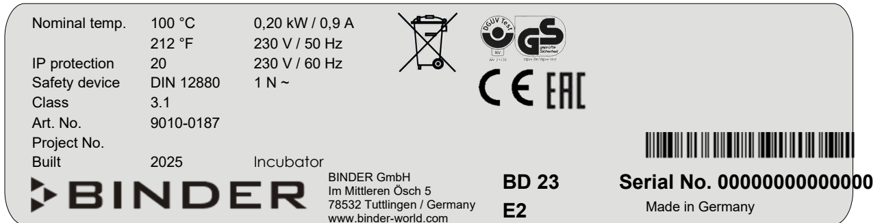
Figure 2: Type plate (example: BD 23 regular chamber)
