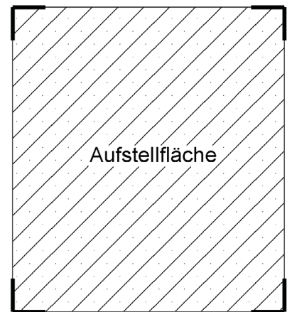
Figure 4: Marking the chamber corners
