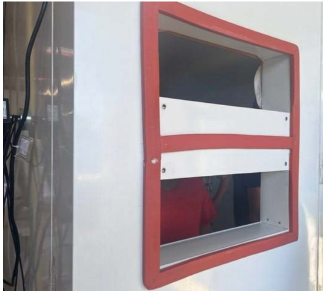
Figure 24: Back of the chamber with silicone gasket at the position of the air conditioner
