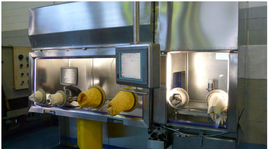
> 1. Isolator module with integrated incubator
