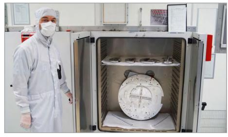
> Components that are used for producing chips must be delivered in an absolutely clean state. BINDER chambers help ensure that every last bit of liquid is removed from the pores.
