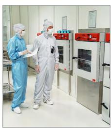
> The vacuum drying chambers from BINDER are used at GEWO to dry components that are used for the production of processors.
