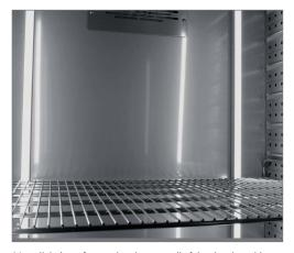
90 cm light bars, fastened to the rear wall of the chamber with tesa Powerstrips  $\ensuremath{\mathfrak{B}}$
