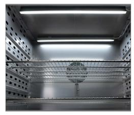
50~cm light bars, fastened to the chamber ceiling with tesa Powerstrips  $\ensuremath{\mathfrak{B}}$
