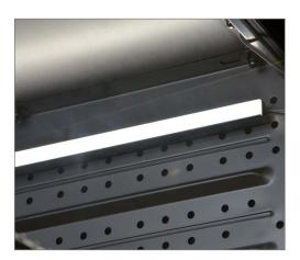
30 cm light bars, fastened to the side of the chamber with tesa Powerstrips  $\ensuremath{\mathfrak{B}}$
