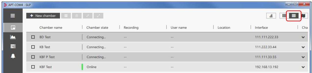
**Active chambers** (meaning a connection exists between controller and APT-COM): These are identified by a green signal and the chamber status “Online” or “Connecting....”
