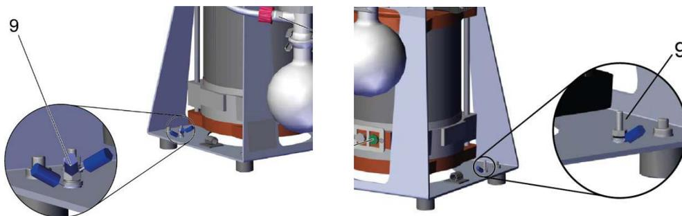
Figure 21: Grounding connections (9) on the pump housing
