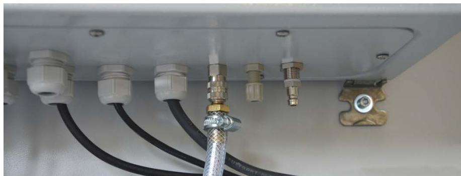
Figure 24: Connection for inert gas at the bottom of the safety module
