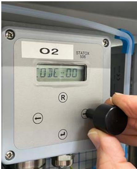
Figure 44: Entering the code for the service menu (example: at the O<sub>2</sub> sensor)
