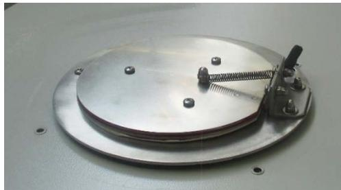
Figure 21: Pressure relief flap at the top of the chamber (delivery condition)
