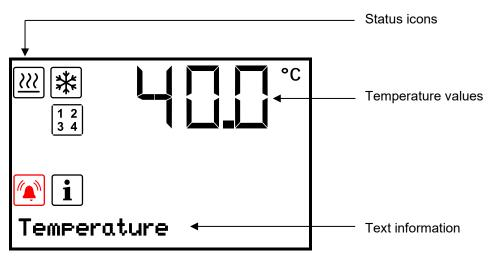
Figure 11: Normal display of the RD4 controller (sample values)
