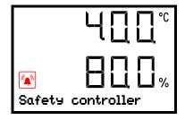
Alarm indication (example: safety controller alarm)
