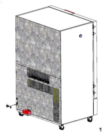
Figure 10: KB ECO 720 with mounted condensate collection pan
