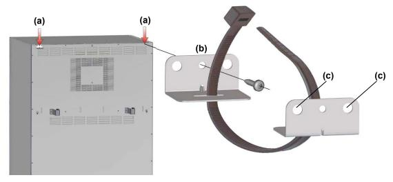
Figure 8: Rear chamber (KB ECO 400) and mounting the flexible tilt protection kit
