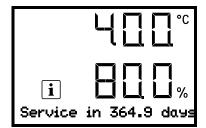
The remaining time in days until maintenance is due is shown in the text field of the controller display.
