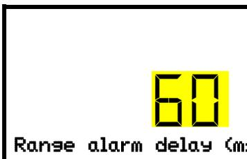
Setting the tolerance range alarm delay.
