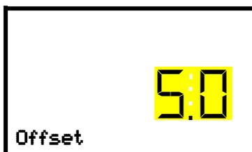
Setting the safety controller value with "Offset" safety controller mode.
