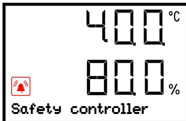
Alarm indication (example: safety controller alarm)
