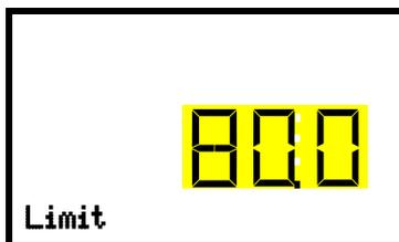
Setting the safety controller value with "Limit" safety controller mode.
