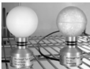
Figure 22: Spherical BINDER sensors for VIS, and UVA measurement
