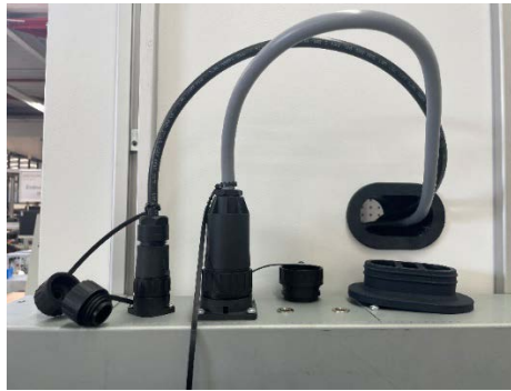
Figure 15: Connections of the light cassettes on the top of the ICH Q1B light box, mounted
