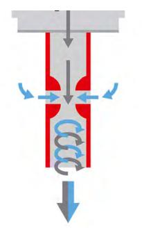
A Venturi nozzle allows for quick atmospheric mixing when CO<sub>2</sub> is injected.
