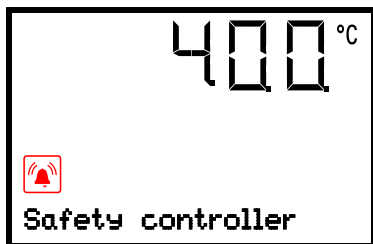
Normal display showing overtemperature safety controller alarm (sample values)
