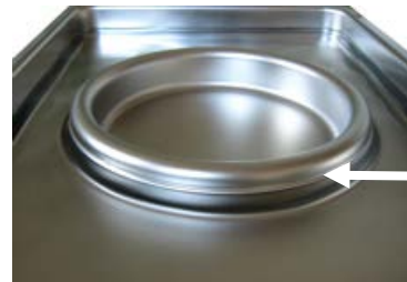
Figure 16: Incubators size 170 / 260, Filling height line of the outer basin
