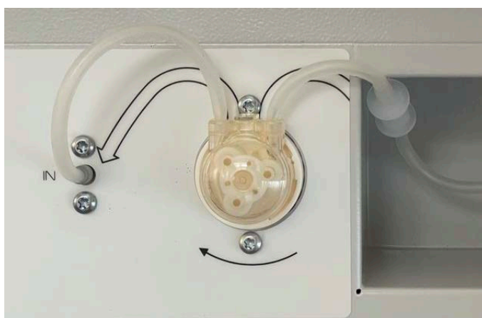
Figure 23: Water supply via freshwater bag, assembled
