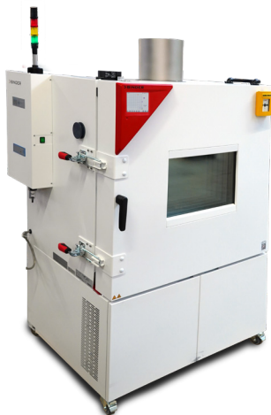
Climate chamber with safety equipment for battery testing
