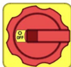
Figure 6: Main power switch (H) in the lateral control panel
