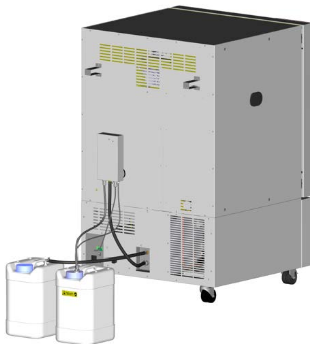
Figure 23: Rear chamber view with external water cans and connections (accessories)
