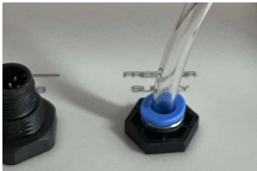
Figure 20: Connecting and disconnecting the ventilation hose
