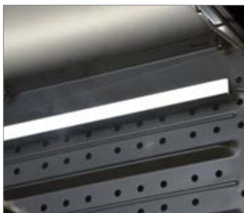
30 cm light bars, fastened to the side of the chamber with tesa Powerstrips®
