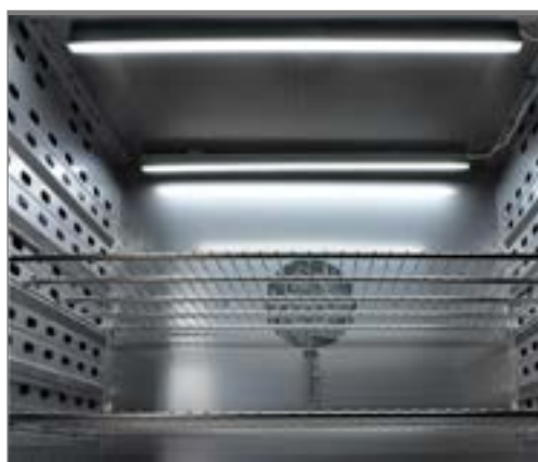
50 cm light bars, fastened to the chamber ceiling with tesa Powerstrips®
