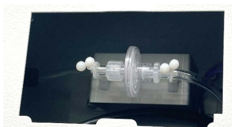
Figure 10: Location of the gas fine filter behind the cover
