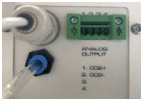
Figure 16: Connecting the CO 2 hose on the CO 2 control box
