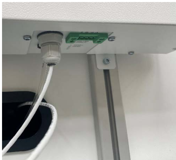
Figure 14: Position of the CO 2 sensor cable with cable gland (9) and access port
