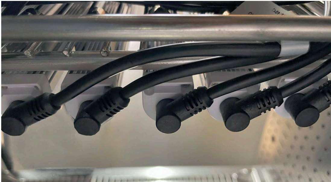
Figure 13: Cable connections to the LED light bars, view from behind
