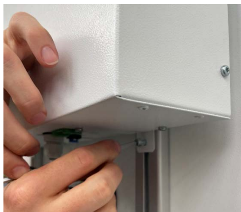
Figure 11: Screwing the plant light box
