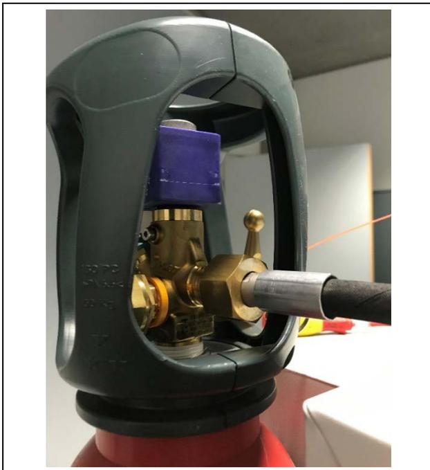
Figure 36: Tuyau haute pression connecté
