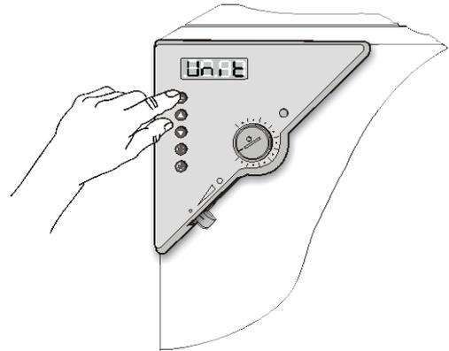
Figure 6: Appuyez sur la touche
