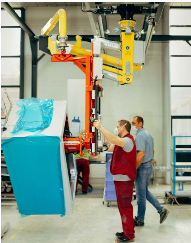
As soon as the housing has been constructed, the chamber is transferred onto the freezer line for further assembly.
