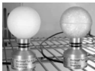
Figure 21: Spherical BINDER sensors for VIS, and UVA measurement
