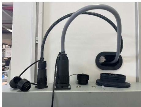
Figure 15: Connections of the light cassettes on the top of the ICH Q1B light box, mounted
