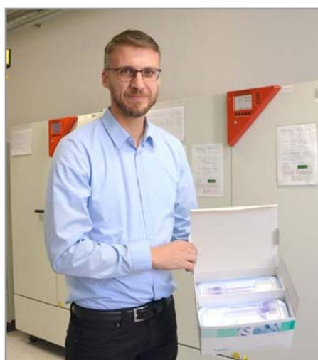
> Trocars and their packaging ready to go into a constant climate chamber for testing.
