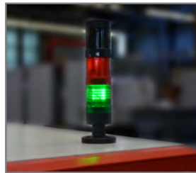
Program sequence display using indicator lamps
