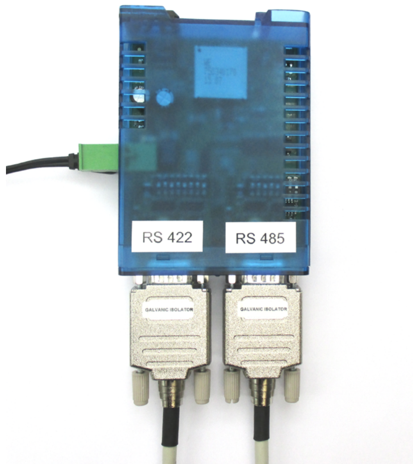
Figure 1: Connected interface converter
